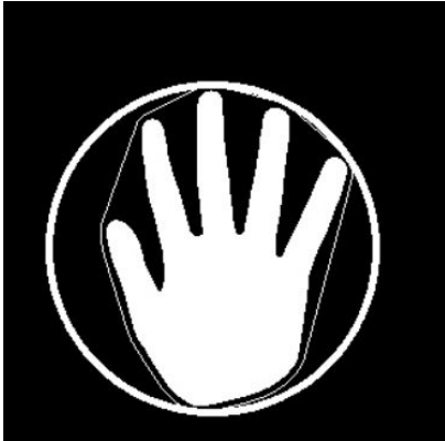
Figure 5: Binary image with detected blob. Bounding circle and convex hull are drawn.
